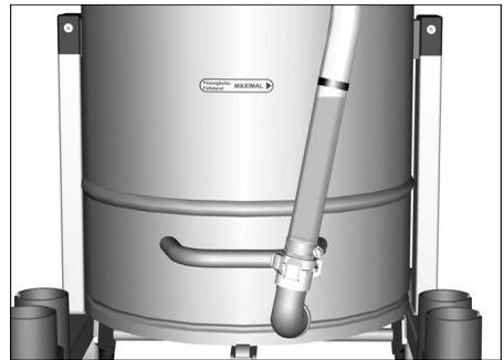
**Note:** The red marking on the drain hose shows the maximum admissible filling level.
